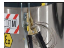
Maximum safety from complete earth grounding of the machine
