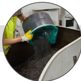
Easily empty swarf from the chip collection basket or from the extractable collection container
