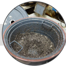
Chip collection basket separates metal chips & oil
